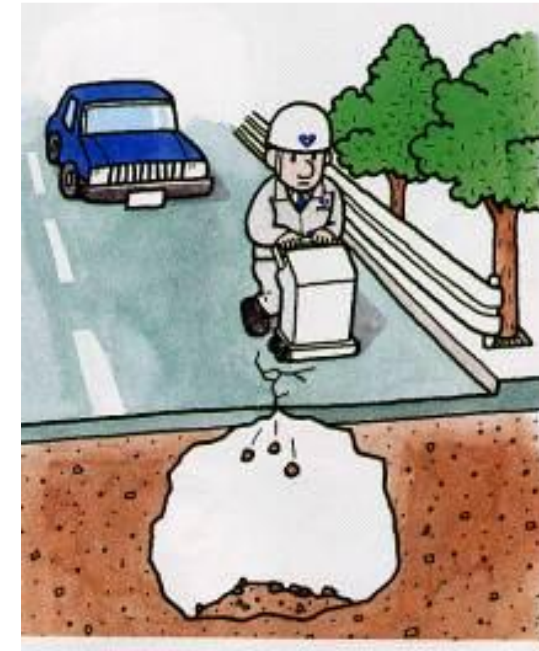
(c). Survey condition under road.
