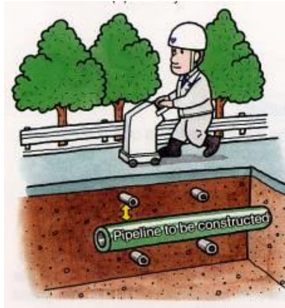
(b). Survey before horizontal drilling
